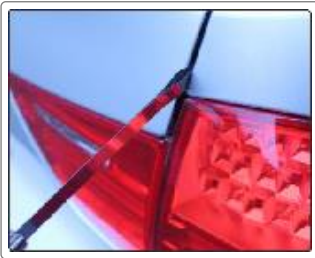
Measuring car body seam
