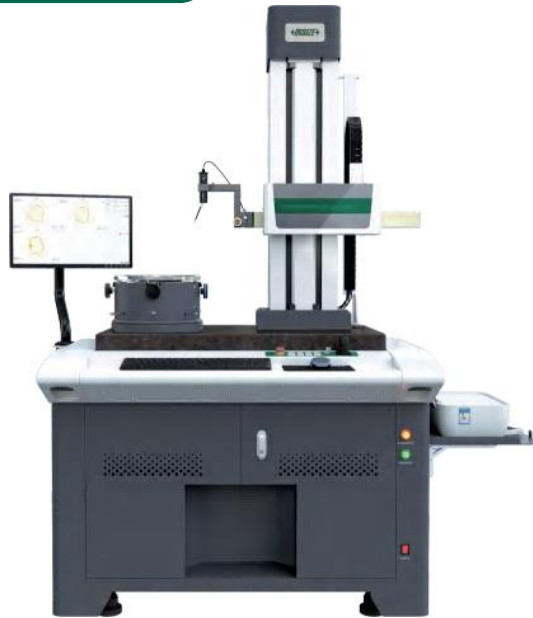
Roundness/Cylindricity Tester RCT-300
