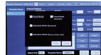
selection of test modes on the calibrator
