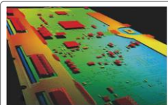
component height measurement on circuit boards
