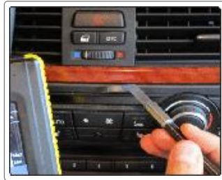
Measuring gaps on the car dashboard
