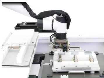
The robot automatically places the workpiece into OK or NG positions on the servo stacking&unloading
